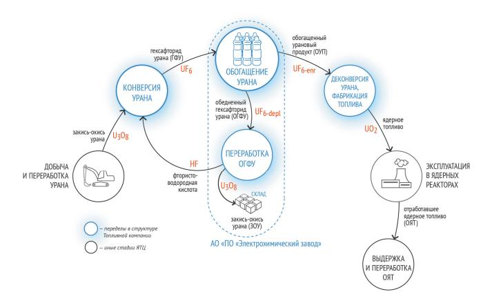
**Production layout of Electrochemical Plant JSC**
