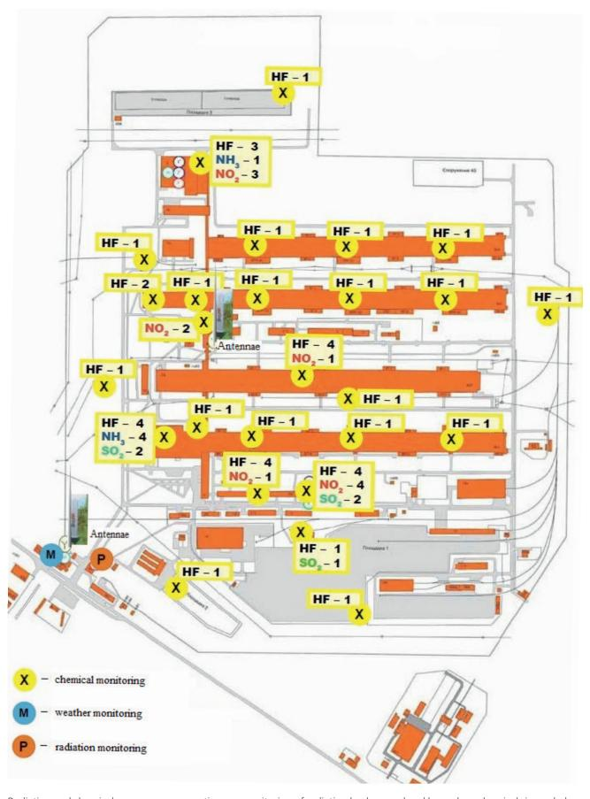
Radiation and chemical sensors ensure continuous monitoring of radiation background and hazardous chemicals in workplace air, within the industrial site, on the border of the sanitary protection zone and in the residential areas of Zelenogorsk.
